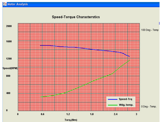
Fig. 9. Screen-shot of Speed-Torque Characteristic of DC Shunt Motor
