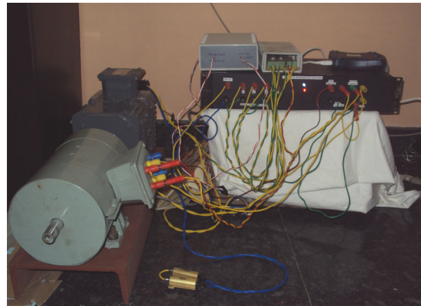
Fig. 8. Practical Set-up for Testing DC Motors
